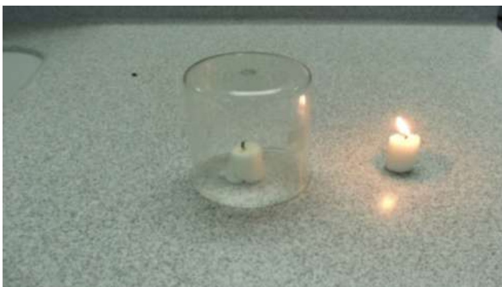
Figure 2: One of the burning candles was covered with Beaker, limiting the access of air to the burning candle.
